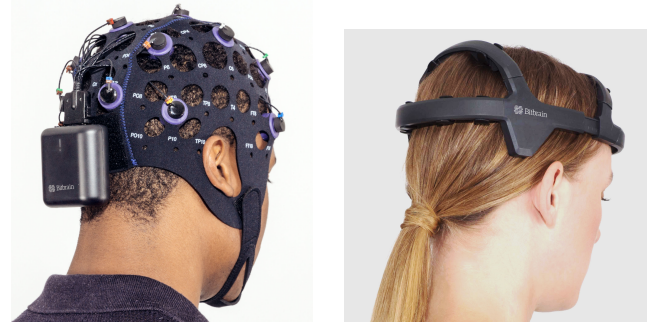
Fig. 1. The two types of portable EEG recording systems. Left) Versatile system with 16 channels and water-based sensors, located on FP1, FP2, F3, Fz, F4, C3, Cz, C4, P7, P3, Pz, P4, P8, O1, Oz and O2. Right) Minimal headset with 12 channels and dry sensors, located on AF7, FP1, FP2, AF8, F3, F4, P3, P4, PO7, O1, O2, and PO8. In both cases the ground and reference electrodes are placed on FPz and left earlobe, respectively.
