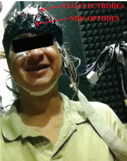
Fig. 1: Combined EEG and NIRS setup
