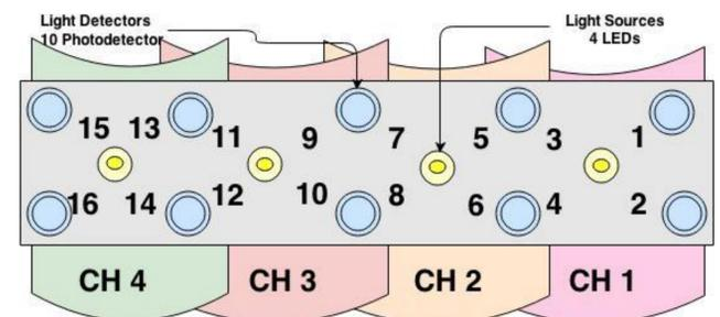
Fig. 2 NIRS Source-Detector Geometry applied to the prefrontal cortex
