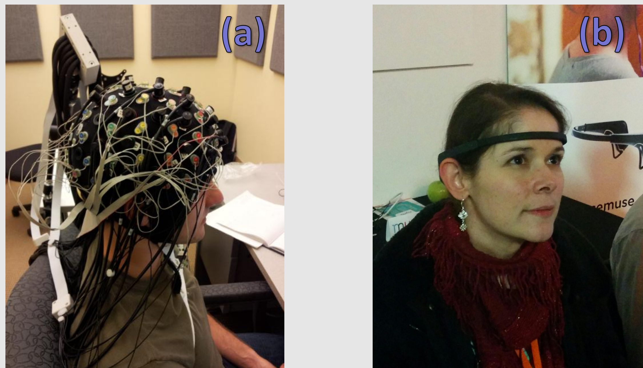
Figure 1. EEG devices (a) Clinical and (b) Consumer grade
